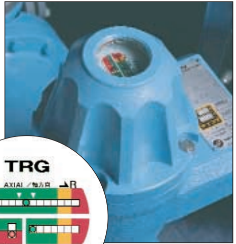
Incorrect rotation is indicated by light at lower left.
